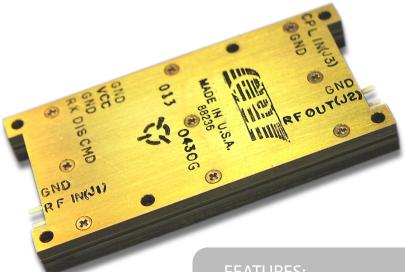
The VLL1871 is a multi-function component consisting of 3 elements: a 40 dB SPST switch, a passive limiter, and a 20 dB directional coupler. All RF ports are coupled through DC blocks.
